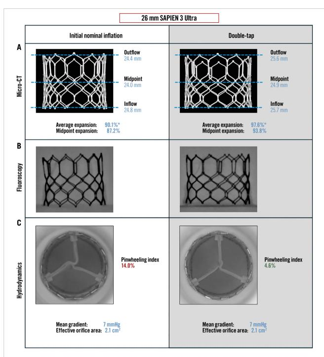
**Figure 1.** Bench assessment of the impact of double-tap on a 26 mm SAPIEN 3 Ultra. Comparison after initial deployment (left column) and following double-tap (right column). THV expansion on micro-CT (A), on fluoroscopy (B), and hydrodynamic function (C). \*Average expansion combining the inflow, midpoint, and outflow areas. Micro-CT: microcomputed tomography; THV: transcatheter heart valve
